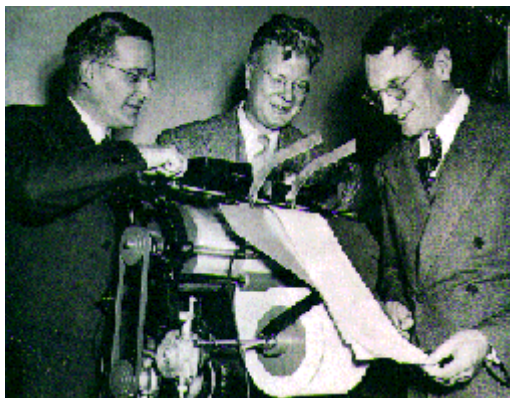
The Xeroxprinter demonstrated in the late 1940s by John H. Dessauer, Haloid's research head; Chester Carlson; and Haloid President Joseph C. Wilson. This early xerographic device, which printed on rolled paper, commanded public attention, but was never marketed as a product.
